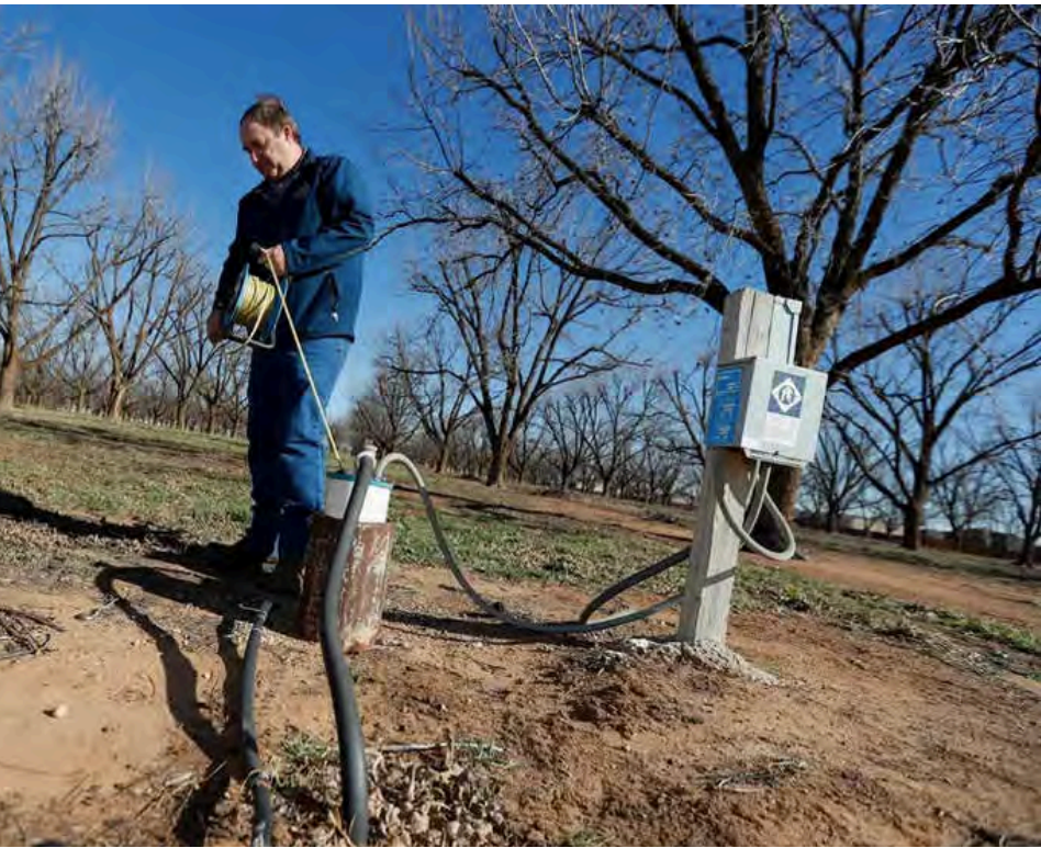
Field Technician Supervisor Billy Barron uses e-line water level meter to check the level of a water well in a pecan orchard in Lubbock County. Barron was checking water levels near the at the High Plains Underground Water Conservation office Friday, Dec. 13, 2023. Photo by Mark Rogers for The Texas Tribune
